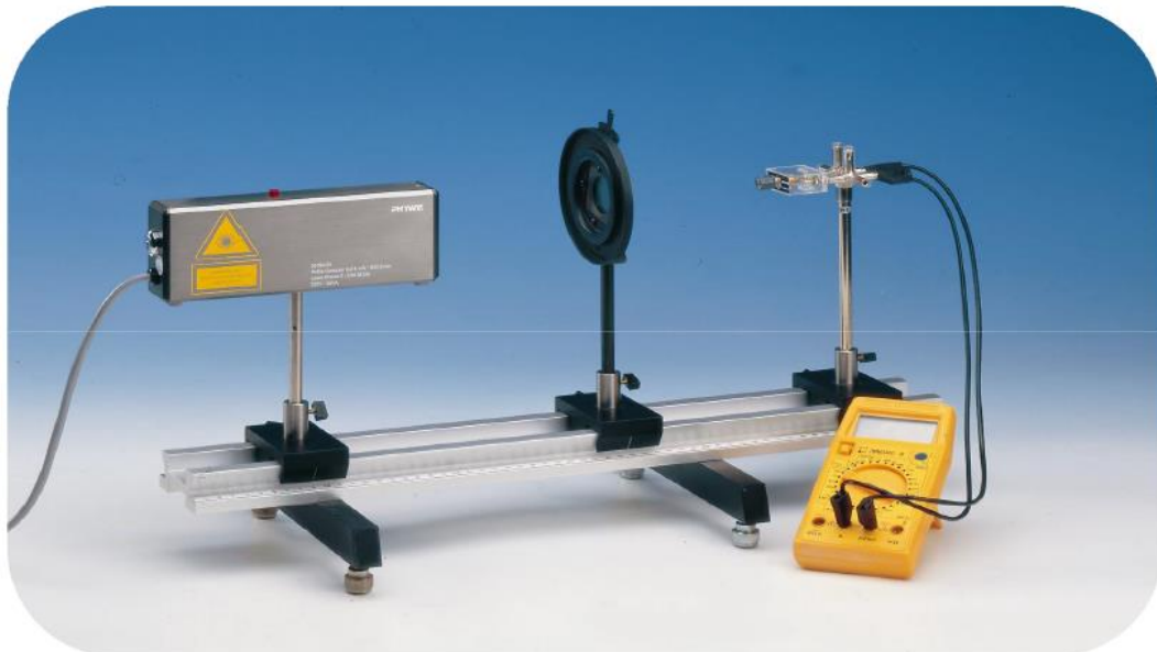
Figure 1: Experimental setup Malus' law
