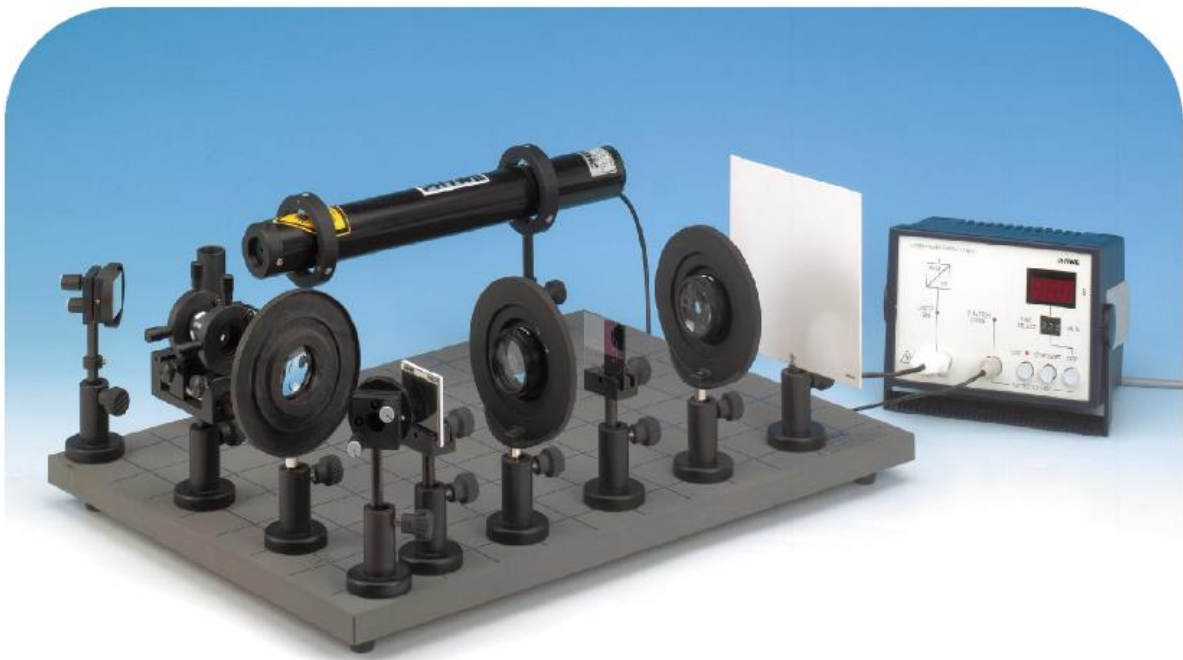
Figure 1: Experimental setup for Fourier optics (4f set-up).
