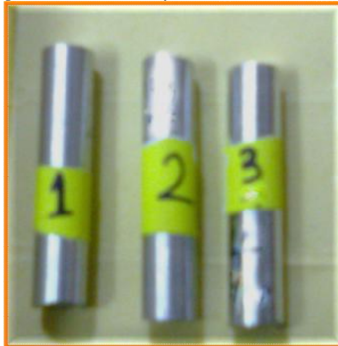
Figure (1-4) Aluminum alloys used in wear test taken for each specimen.
