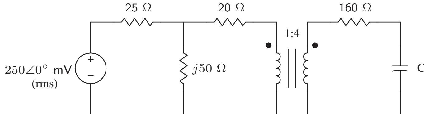
Find the value of  $C$  that maximizes the power absorbed by the  $160 \Omega$  resistor. What is the average power delivered for this value of  $C$ ? Replace the resistor with a variable resistor and find the value that maximizes the power delivered? What is the maximum average power that can be delivered?
