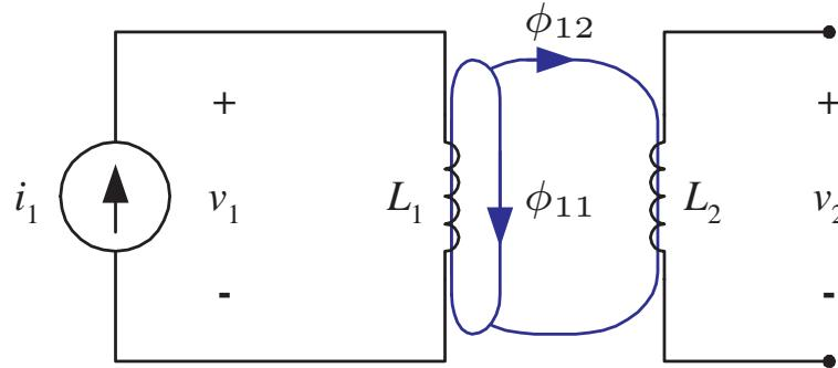
$$v_1 = L_1 \frac{di_1}{dt} \quad v_2 = \pm M_{21} \frac{di_1}{dt} \quad M_{21} = N_2 N_1 \mathcal{P}_{12}$$
