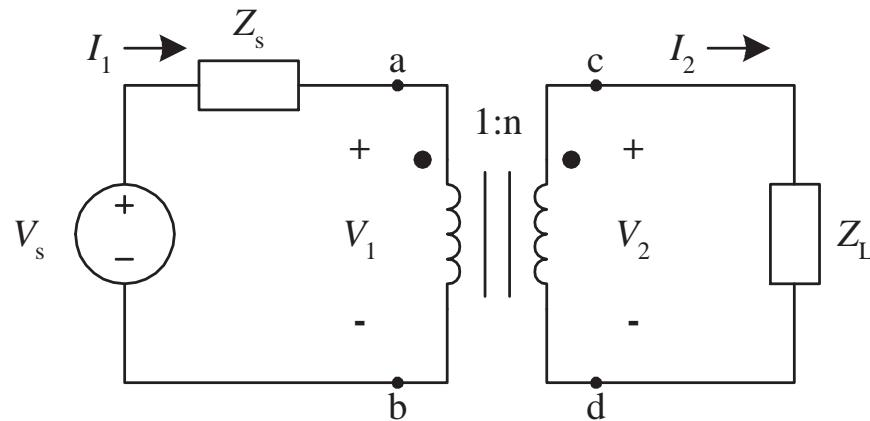
$$Z_R = \frac{V_1}{I_1} = \frac{V_2 \frac{1}{n}}{I_2 n} = \frac{V_2}{I_2} \frac{1}{n^2} = \frac{Z_L}{n^2}$$
