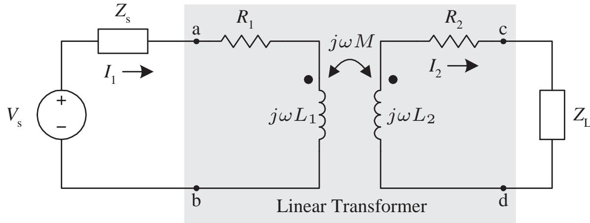
$$Z_{ab} = R_1 + j\omega L_1 + \frac{\omega^2 M^2}{Z_{22}}$$
