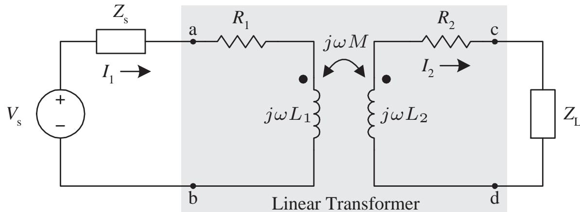
$$V_s = (Z_s + R_1 + j\omega L_1)I_1 - j\omega M I_2$$
