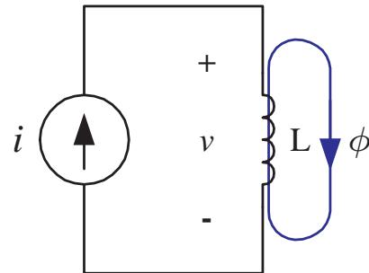
$$v = N \frac{d\phi}{dt} = (N^2 \mathcal{P}) \frac{di}{dt} = L \frac{di}{dt}$$
