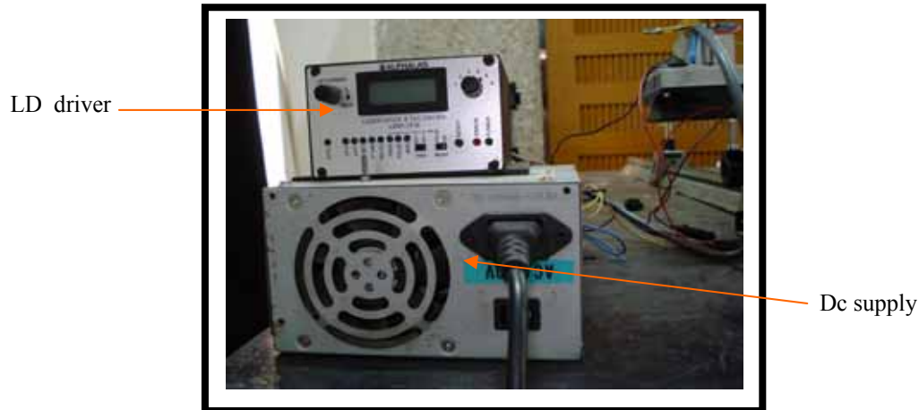
Fig.(4.2) the laser diode driver with its external power supply.
