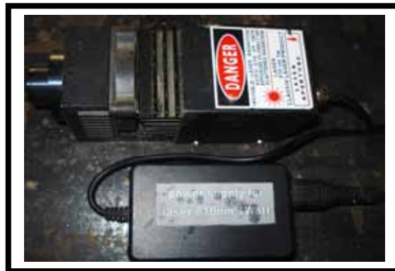
Fig.(4.4) QW CW 810 nm GaAlAs laser diode.
