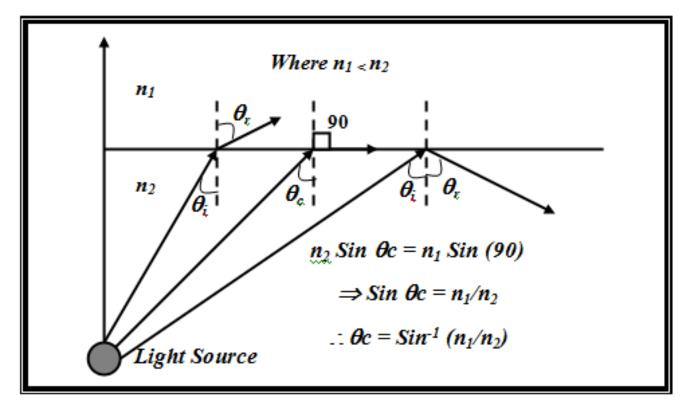
Figure (1.3) the Total Internal Reflection[5]
