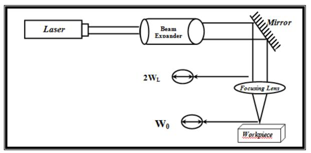
Figure (1.4) Schematic layout of a laser beam delivery[4]
