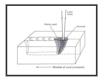
Figure (2.2) formation of a "keyhole" during high power laser welding[4]
