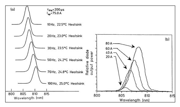
Fig.3 (a) Diode array linewidth vs. repetition rate and (b) wavelength shift vs. drive current
