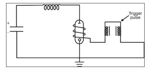
Fig. 2 External trigger circuit
