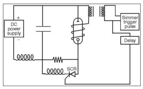
Fig. 8 Circuit for pseudosimmer mode operation
