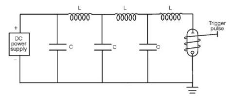
Fig. 6 Multiple-mesh discharge circuit
