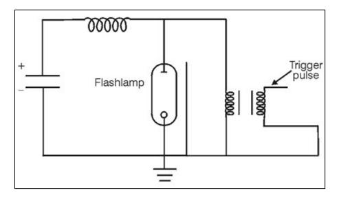
Fig. 4 Parallel trigger circuit
