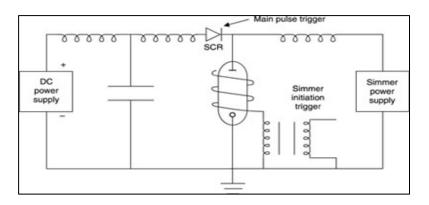
Fig. 7 Circuit for simmer mode operation
