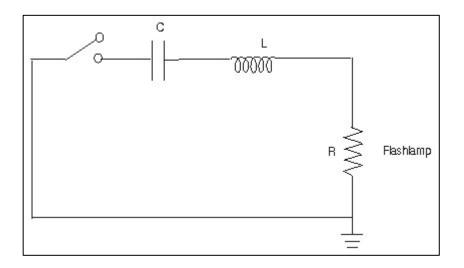
Fig. 5 RLC discharge circuit
