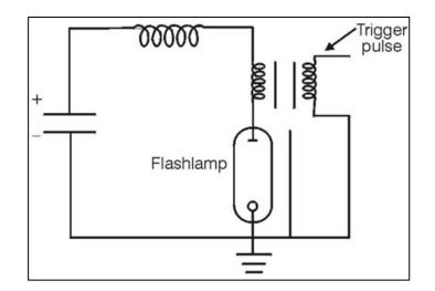
Fig. 3 Series trigger circuit
