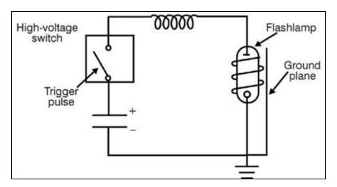
Fig. 1 Over voltage trigger circuit
