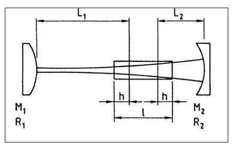
Concave-convex resonator containing a Nd:YAG rod
