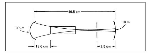
Fig.2 Focusing resonator geometry
