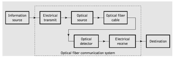
Figure 1.5: Optical fiber communication system.
