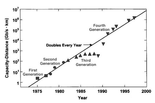
Figure 1.3: Increase in the BL product over the period 1975 to 1980 through several generations of lightwave systems. Different symbols are used for successive generations.
