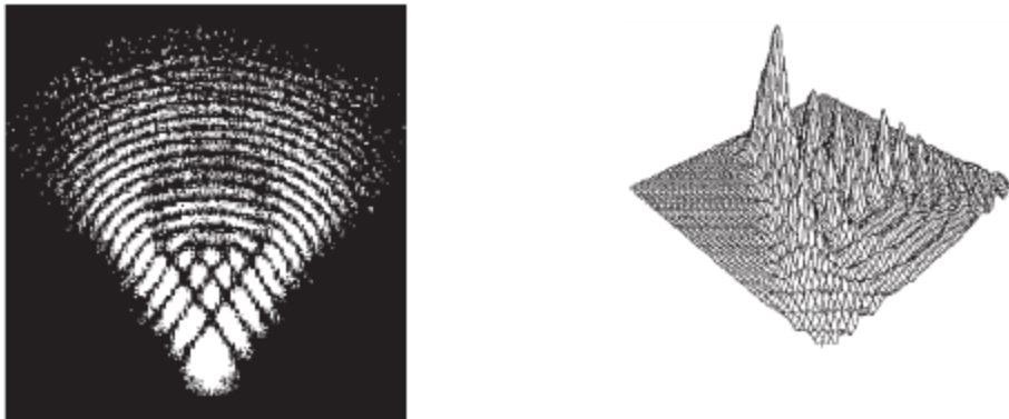
Figure 6.24 Third-order coma. (a) A computer-generated diagram of the image of a point source formed by a heavily astigmatic optical system. (OPAL Group, St. Petersburg, Russia.) (b) A plot of the corresponding irradiance distribution. (OPAL Group, St. Petersburg, Russia.)
