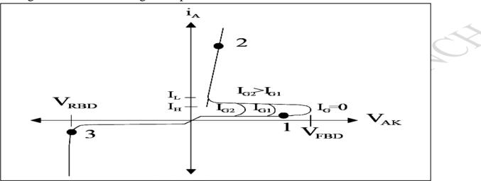
The thyristor moves rapidly along the negatively sloped portion of the curve until it reaches a stable operating point determined by the external circuit (point "2"). The portion of the graph indicating forward conduction shows the large values of  $i_A$  that may be conducted at relatively low values of  $V_{AK}$ , similar to a power diode.
