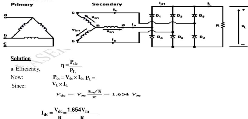
$V_L = V_m \sqrt{\frac{3}{2} + \frac{9\sqrt{3}}{4\pi}} = 1.655 V_m$  $I_L = \frac{V_L}{R} = \frac{1.655V_m}{R}$  $\eta = \frac{(1.65V_m)^2 R}{(1.655V_m)^2 R} = 99.85\%$  $FF = \frac{1.655V_m}{1.654V_m} = 1.0008$
