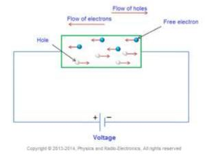
In a semiconductor, the electrons always try to move in a straight line towards the positive terminal of the battery. But, due to continuous collision with the atoms they change the direction of flow. Each time the electron strikes an atom it bounces back in a random direction. The applied voltage does not stop the collision and random motion of electrons, but it causes the electrons to drift towards the positive terminal.
