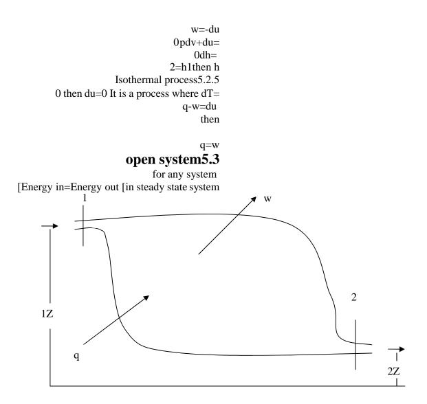
$q + flowwork_{in} + (potential + kinetic + int ernal)Energy_{in} =$  $w + flowwork_{out} + (potential + kinetic + int ernal)Energy_{out}$
