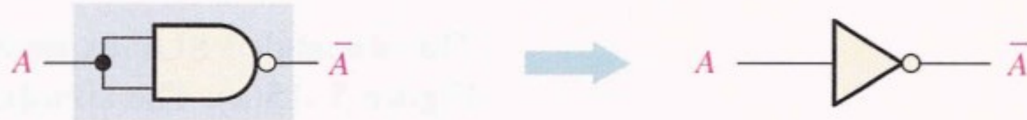
(a) One NAND gate used as an inverter
