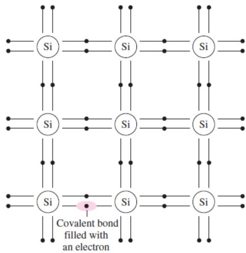
The outer shells of the silicon atoms are full, and the material behaves as an insulator. As the temperature increases, thermal energy is added to the crystal and some bonds break, freeing a small number of electrons for conduction, a
