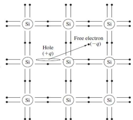
The density of these free electrons is equal to the intrinsic carrier density ni (cm<sup>-3</sup>), which is determined by material properties and temperature:
