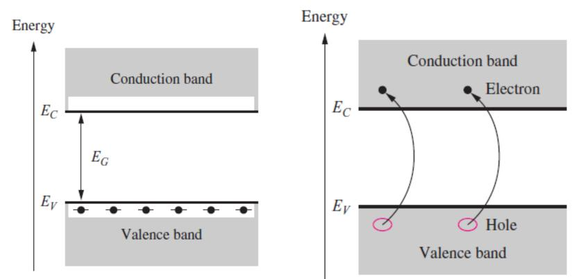
Semiconductor at 0 K with filled valence band and empty conduction band.
